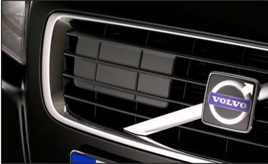
The radar sensor in this Volvo's grill is part of the Collision Warning and Auto Brake system.
